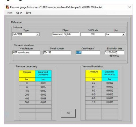
On this page are stored all data on standard instruments that can be used during the calibration.
