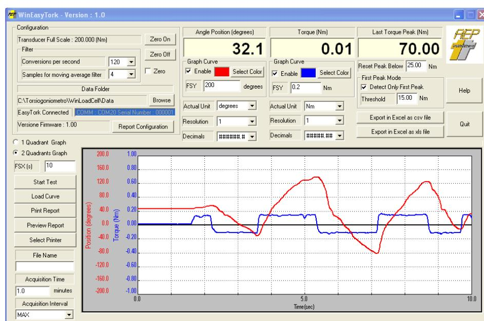
The Software allows you to directly manage the torque of the series **EasyTORK**, displaying real-time measurement of TORQUE and ANGLE or alternatively the SPEED of rotation (in Hz or rpm).
