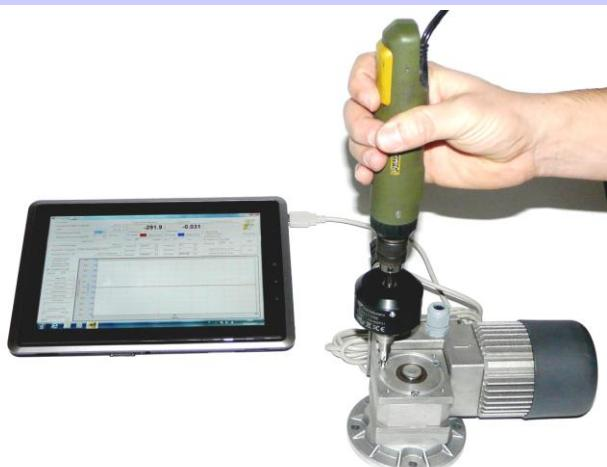
Rotating torque transducers for measurements TORQUE and SPEED ANGLE both under static and dynamic conditions in continuous rotation. The sensors of this series are used in various measurement applications, associated with processes of calibration, quality control in laboratories and in industrial applications where it is necessary to check:
