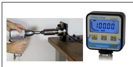
DTR2 + TRF STATIC Torsiometer. System for calibrating impact wrenches
